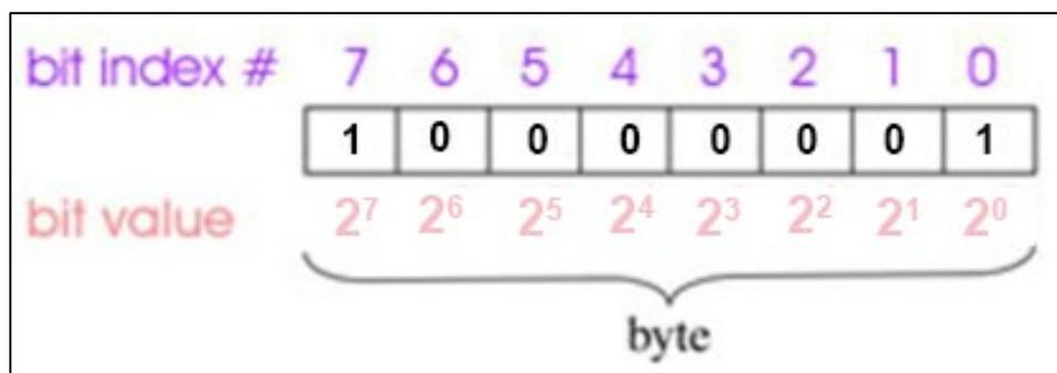
Figure 1. This figure shows the bit flag format. The bit index positions are numbered from right (bit index 0) to left (bit index 7), and each index stores the result of a screen test. The bit values from right to left solve respectively to 1, 2, 4, 8, 16, 32, 64, and 128. In this example, bit index 0 and bit index 7 are set to true (1) with corresponding bit values 20 and 27 equaling '1' and '128', which when summed equal '129'.
