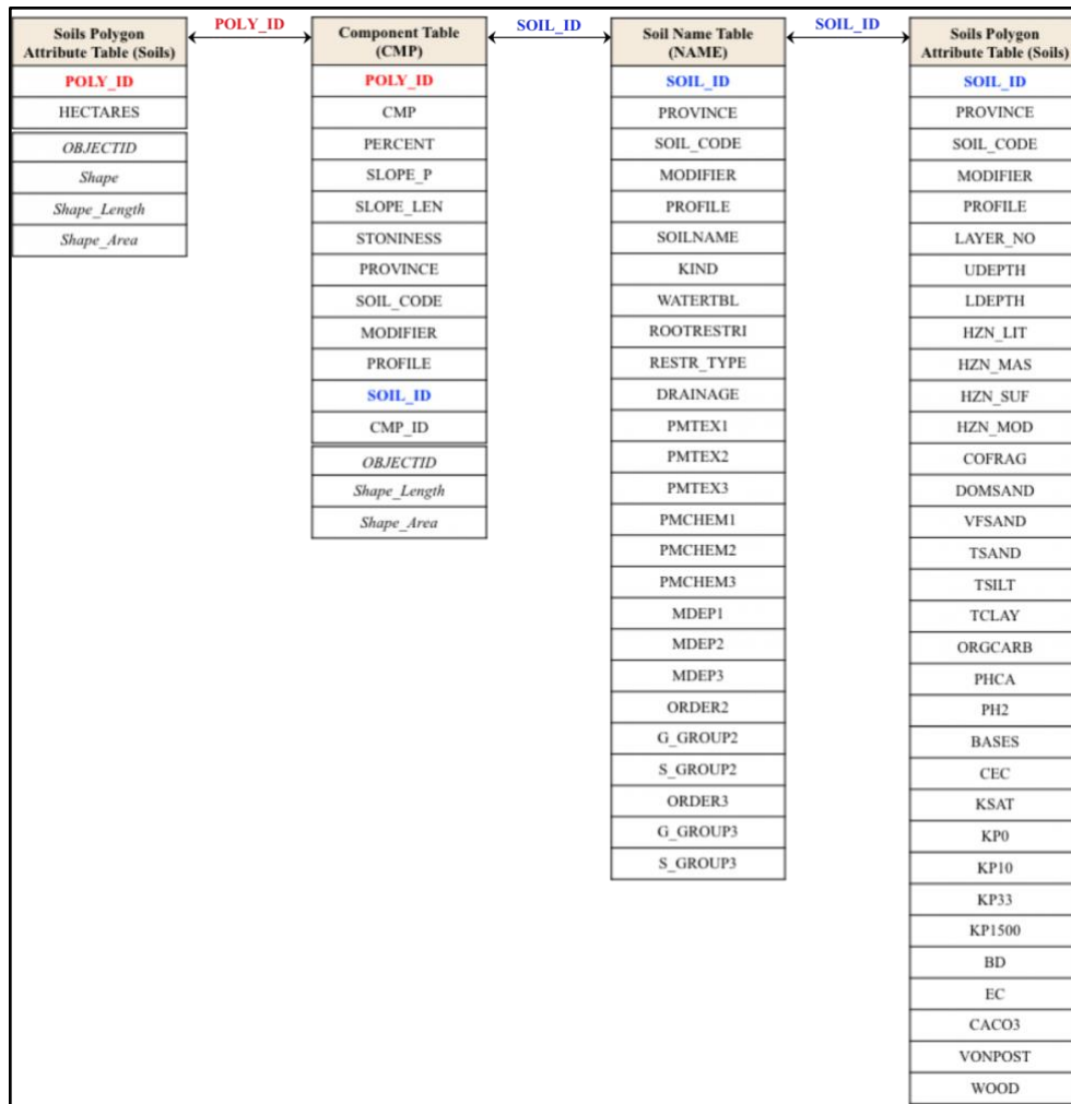
Figure 2. The Soils polygon and CMP table can be joined through their shared POLY_ID fields (in red). The CMP table can also be joined to the NAME and LAYER tables through their shared SOIL_ID fields (in blue). Within each feature class's table, italicized fields are specific to ArcGIS and do not represent soil classification.
