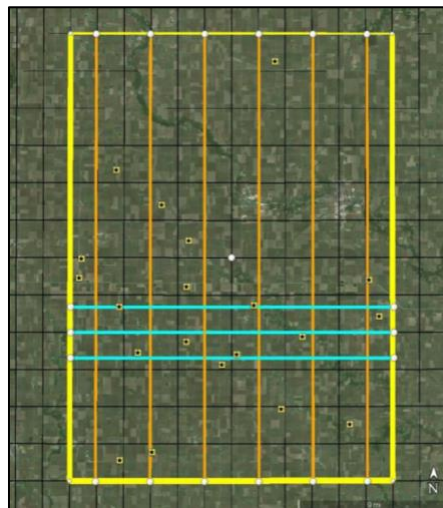
Figure 2. Example of PALS flight lines drawn on Google Earth. High-altitude (3000 m) mapping lines are marked with orange and the low-altitude (1200 m) high resolution lines are marked with light blue.
