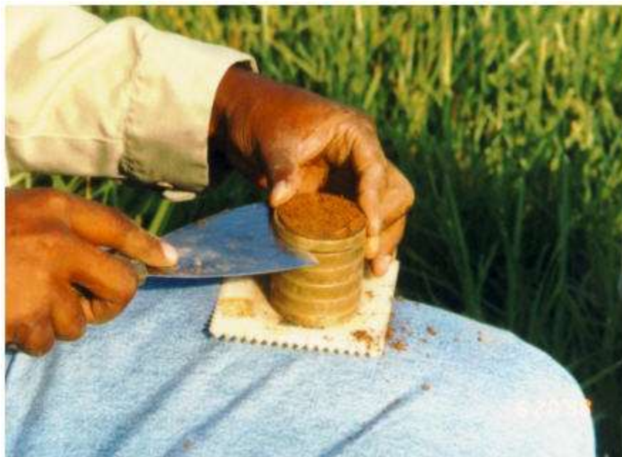
Figure 1: Demonstration of the Sliced Core Sampling Technique
