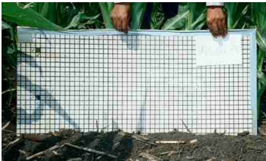
Figure 1. Measuring Board Used to Photograph Surface Roughness
