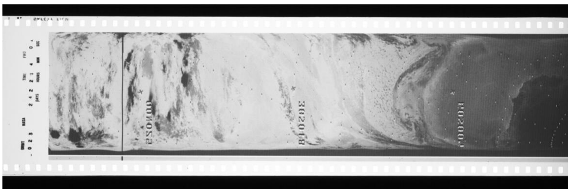
Figure 1. This figure shows grayscale radiative temperatures from Nimbus 1, orbit 023, acquired on August 29, 1964. The satellite orbit and observation date and time are burned into the left margin of the film and latitude/longitude coordinates are burned into the image. Note, this metadata may not be included in all images.
