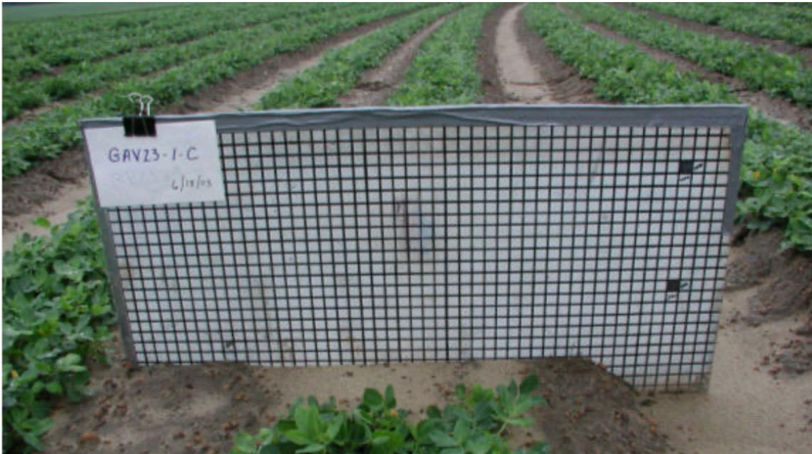
Figure 2 A grid board used for surface roughness measurements during the SMEX03 campaign.
