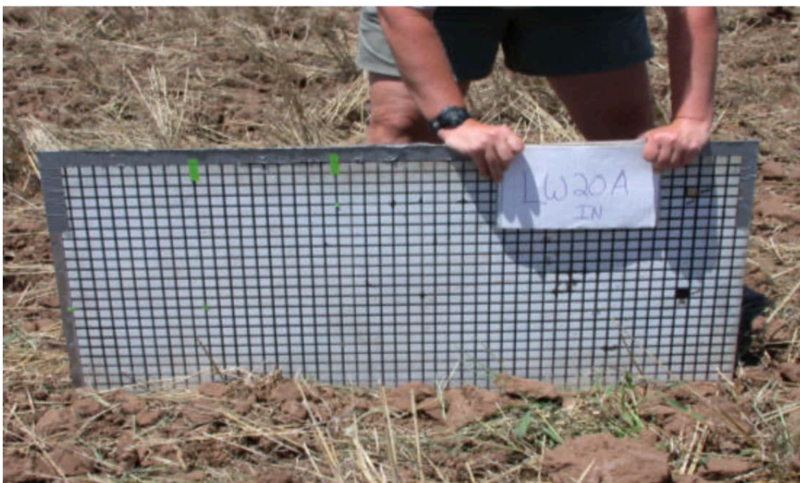
Figure 3 A grid board used for surface roughness measurements during the SMEX03 campaign.
