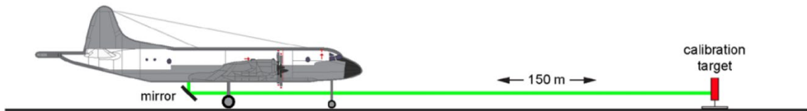
Figure 4. Range bias determination (a.k.a. ground test) using a calibration target with a known distance. The distance to the calibration target is measured with an electronic distance meter (a.k.a. total station) with an accuracy of a few millimeters.
