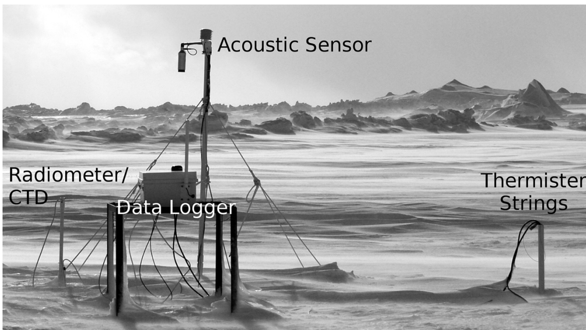
Figure 4. IMB buoy deployment. The IMB buoy is not visible from the top side of the ice. Photograph courtesy of M. Lewis. Click for larger view.
