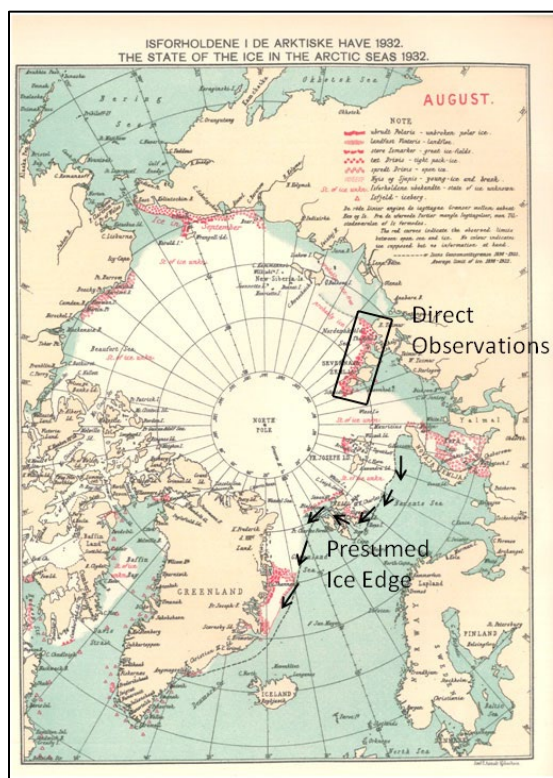
Figure 1. An August 1932 example from the DMI Arctic Sea Ice Charts data set. Ship and shore observations are marked in red. The presumed, but not observed ice extent, is the white field. Observed regions may often show the type of ice present using a legend in the top right corner.
