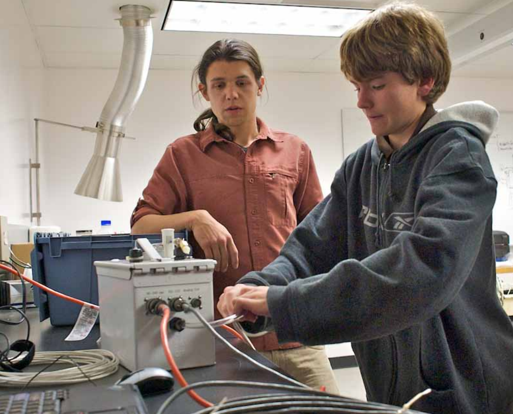
NOAA's Ryan Neely watches young scientist Hunter Solheim put together his instrument, an infrared thermometer that can monitor cloud-bottom conditions. Photo by Will von Dauster, NOAA.
