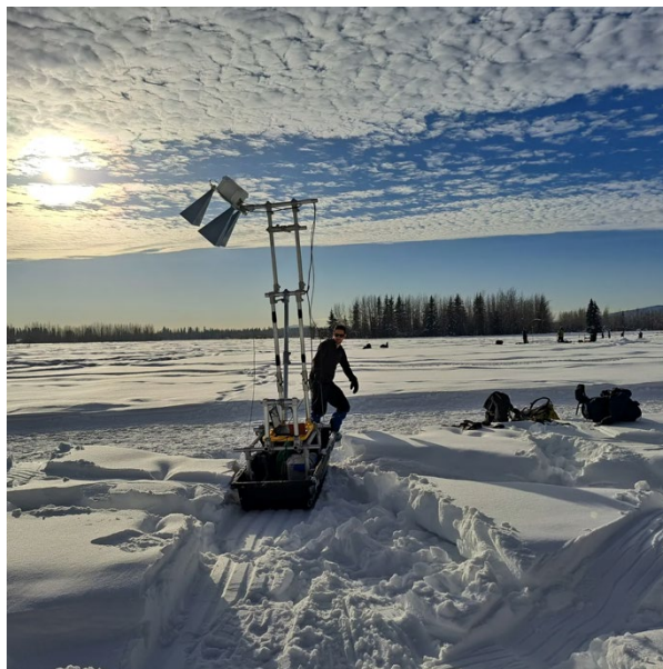
Figure 1. Sled-mounted tower-based radar system being towed along a transect.
