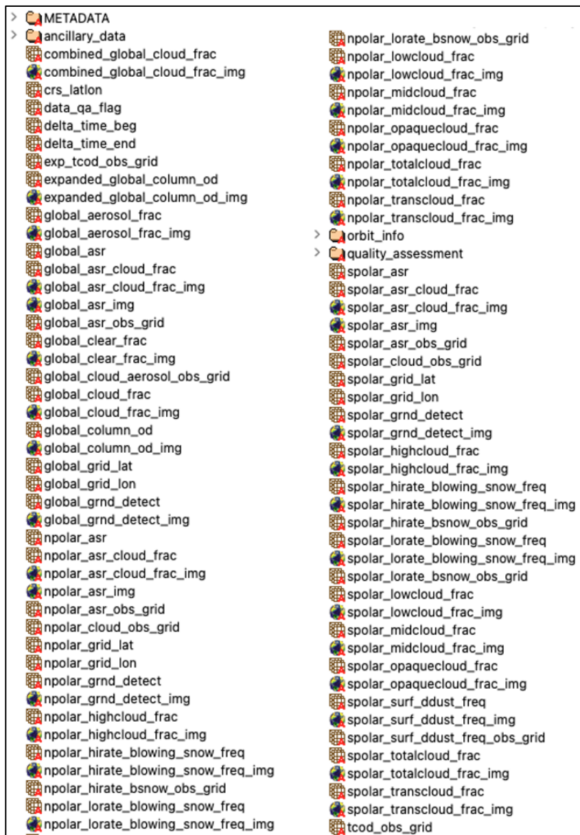
Figure 1. Internal structure of an ATL16 data file. ATL17 data files utilize the same structure and variable names.
