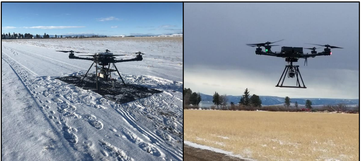
Figure 1. Freefly Alta X UAV with Riegl miniVUX-2 LiDAR system used for snow-on acquisitions.
