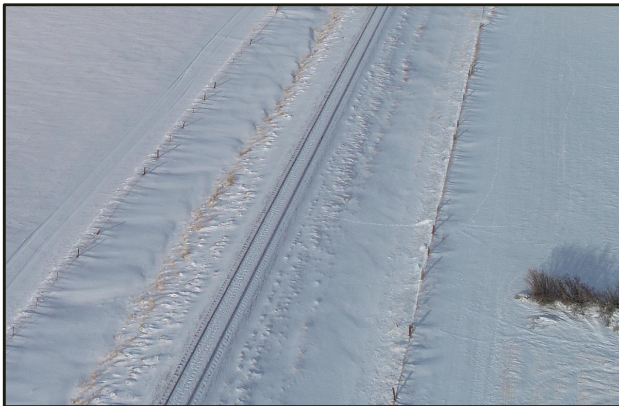
Figure 31. Aerial photo of train tracks taken on 2/18 showing presence of snow on railroad ties. The elevation difference caused by this snow cover is observable in the 2/17 and 2/18 snow-on point clouds.
