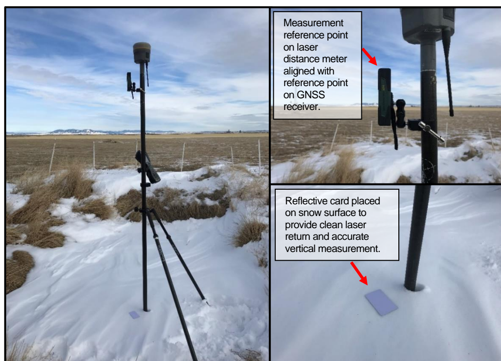
Figure 5. A Trimble R10 GNSS receiver mounted on a survey rod equipped with a laser distance meter. By placing a reflective card on the snow surface, an accurate instrument height measurement to the snow surface could be obtained.
