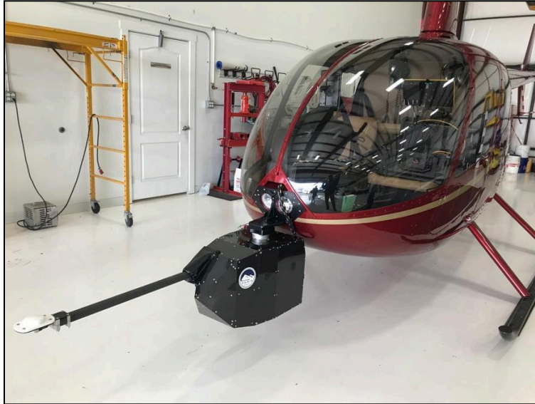
Figure 2 - CRREL's nose-mounted Meeker System installed on a Robinson R66 helicopter. All sensors are located inside the pod, with control systems located within the passenger compartment for in-flight operations.
