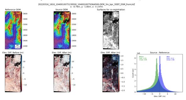
Secondary vertical-only translation (constrained to manually identified control surfaces):
