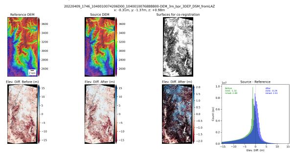
Secondary vertical-only translation (constrained to manually identified control surfaces):
