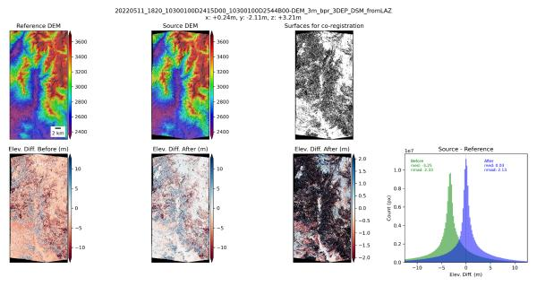
Secondary vertical-only translation (constrained to manually identified control surfaces): Secondary z shift applied: +0.13 m
