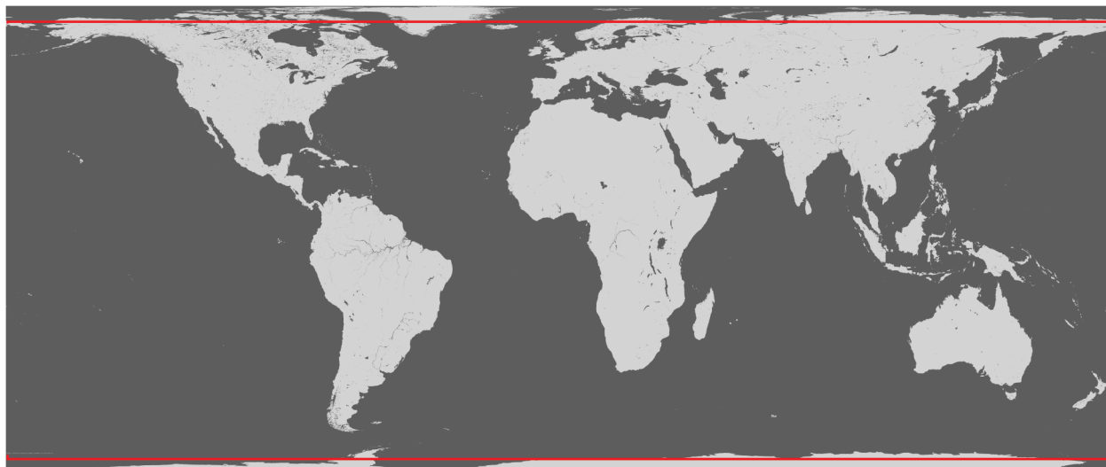
Figure 2: Cylindrical EASE-Grid 2.0 projection extents. Full extent coverage is EASE2-M, with horizontal red lines delineating the smaller latitudinal extent of EASE2-T grid. Land-ocean mask from Brodzik and Knowles (2011).
