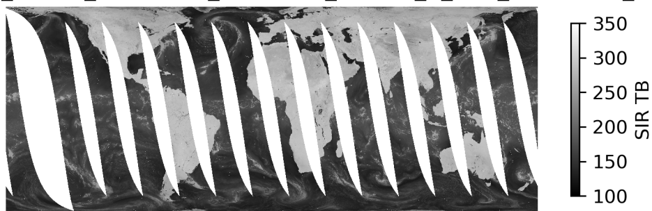
Figure 22: CETBv2 Cylindrical AMSR2 ascending pass 36H GRD 25 km (top) and rSIR 3.125 km (bottom) brightness temperatures, 30 Apr 2023.
