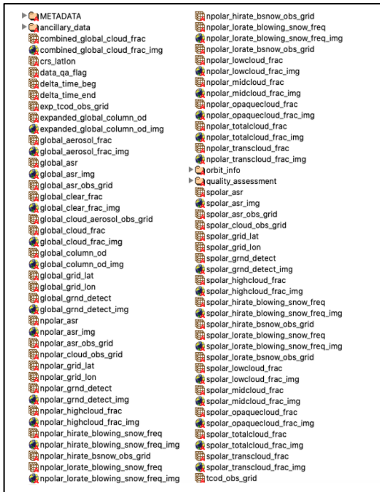
Figure 3. Internal structure of an ATL16 data file (Left: top half; Right: bottom half). ATL17 data files utilize the same structure and variable names.
