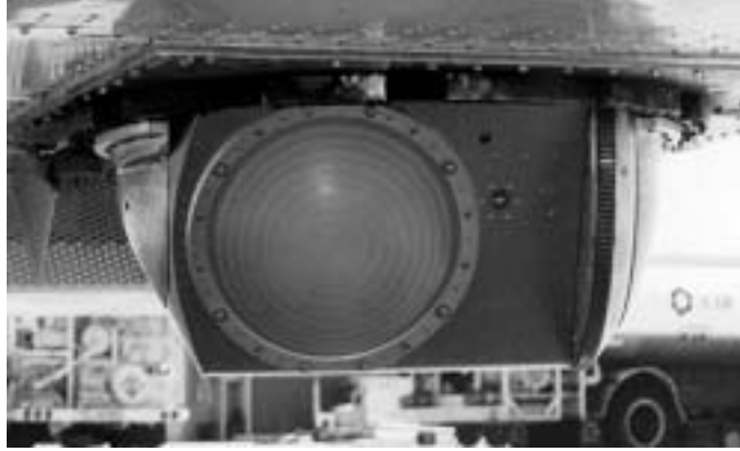
Figure 3. PSR/C scanhead installed on the NASA P3-B aircraft during the SGP99 experiment.
