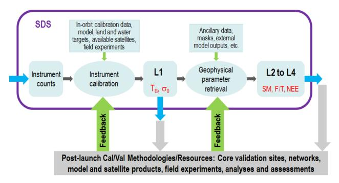
Figure 2.1. Overview of the SMAP Cal/Val Process.
